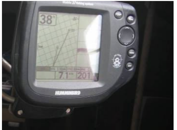
the GPS linked depthsounder, fish finder, speed gauge and compass
